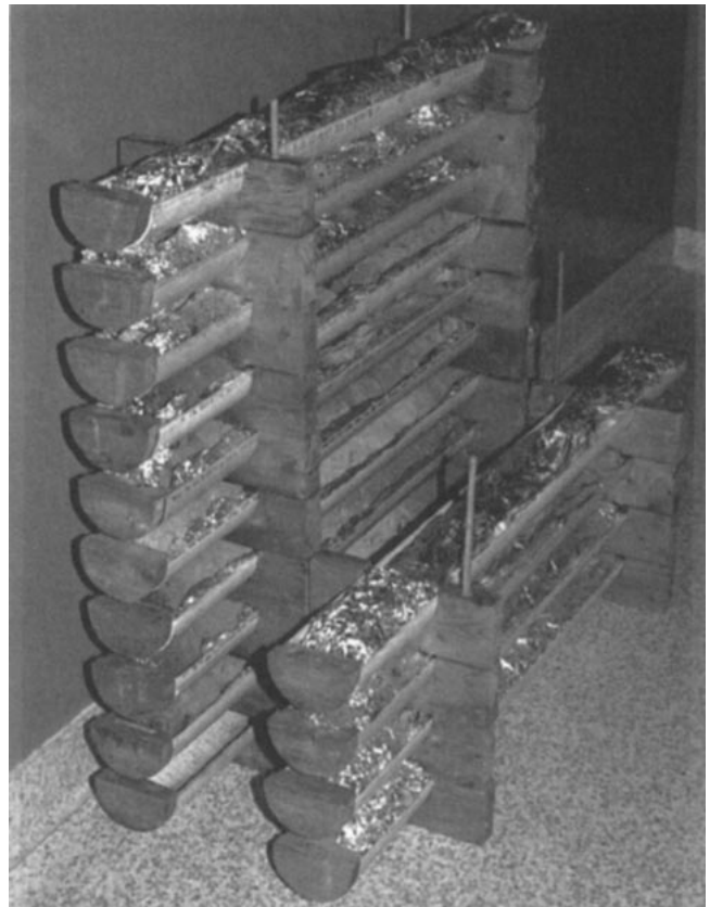
Fig. 3. A stack of soil trays stabilized by wooden dowels. Trays filled with soil cores can be stacked at least 10 high using dowels.
