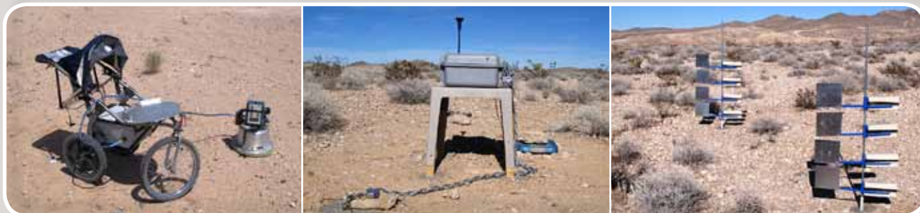
Some of the devices used to collect data in the NDRA study (left to right): PI-SWERL (Portable In Situ Wind Erosion Laboratory), DustTrak (used to measure PM10 concentrations), and BSNE (Big Spring Number Eight) dust traps. Photos by Dr. Dirk Goossens, UNLV.
