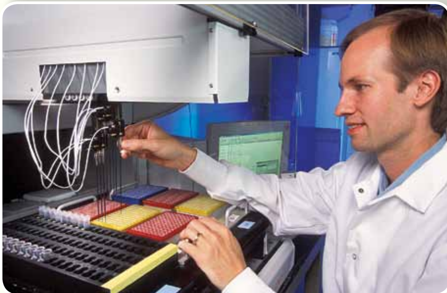
Plant geneticist Edward S. Buckler uses high-throughput robotics to efficiently sample the DNA variation of thousands of genes in maize. Photo by Peggy Greb (USDA-ARS).
