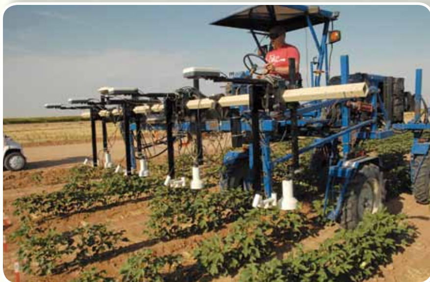
In Arizona, Michael Gore, Pedro Andrade-Sanchez, and John Huen are working on tractor-based proximal remote sensing. This high-throughput phenotyping system is being used to collect plant height, canopy temperature, and canopy reflectance data from cotton plants. Phenotyping is still very expensive so the group hopes that strategies such as this will lower the costs. Photo courtesy of Michael Gore.
