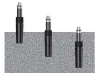
Measuring CO 2 in soil using the GMT220 probe
