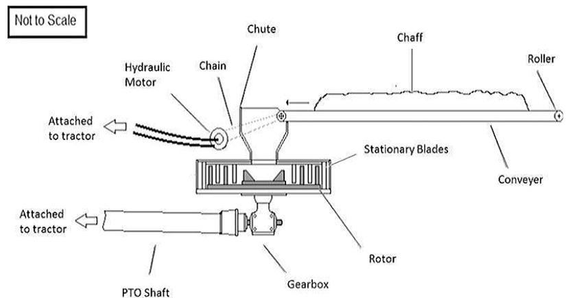
The integrated Harrington Seed Destructor (iHSD) utilizes the tractor’s hydraulic system to feed chaff into a chute where rotating blades grind crop residue into a fine powder, erasing seed viability. Watch the iHSD in action here: [https://youtu.be/MU-atcUQ\\_ZI](https://youtu.be/MU-atcUQ_ZI).
