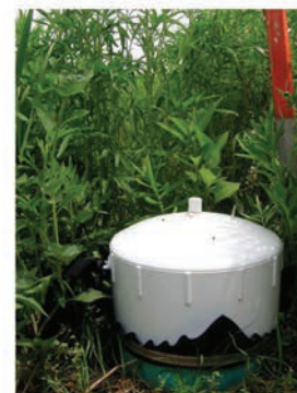
Static chamber for greenhouse gas measurements.
