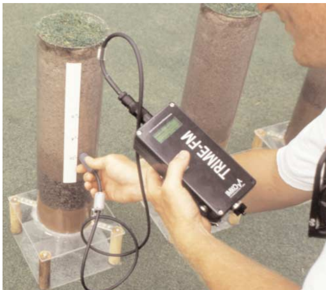
Fig. 3. Student measuring water content of soil column with time domain reflectometry (TDR) probe.
